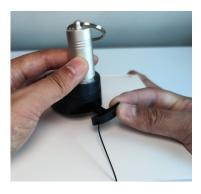
**3. Remove Locking Clip**Once the Locking Clip is released from the Main Housing, pull out completely.
