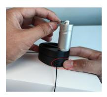
2. Push Locking Clip in to Release Gently push in the Locking Clip into the Main Housing until you hear a faint click.
