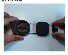
Wind up the Cables so the Medallion is engaged with the Main Housing.
