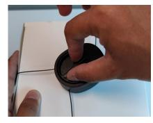
4. Tighten Cables around merchandise Lift and turn the Flip-Up Winder clockwise to snugly tighten the Cables around the merchandise (an audible clicking noise will be heard). installation process.
